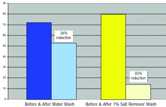
The existing coating was in acceptable condition for overcoating; power tool cleaning was specified with blasting only being done at the beam ends under the joints. Washing was a preliminary step before power tool cleaning. The tests were performed over corroded areas before power tool cleaning.
